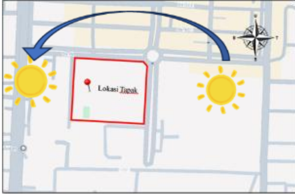
Figure 9. Sunlight Analysis – the eastern portion of the site receives strong morning light, prompting the placement of shade trees as solar filters.
